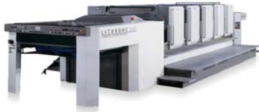
국반절 4색기 KOMORI LITHRONE 28 Offset Printing Press 15,000 tph Printing speed
