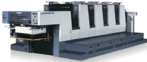
국반절 4색기 KOMORI LITHRONE 28 Offset Printing Press 15,000 tph Printing speed
